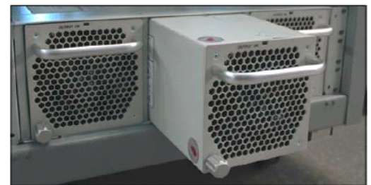
Power Supply Module in Chassis
